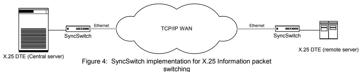
This packet-switching approach allows designers to use the SyncSwitch and an IP infrastructure to replace both leased lines and the packet-switching network, as illustrated above in Figure 4. Although there are no performance benefits to the end devices, sensitivity to IP network performance is greatly reduced, as the SyncSwitch both buffers information and responds immediately to legacy device protocol sequences.
