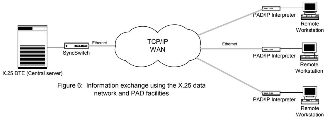
Figure 6: Information exchange using the X.25 data network and PAD facilities
