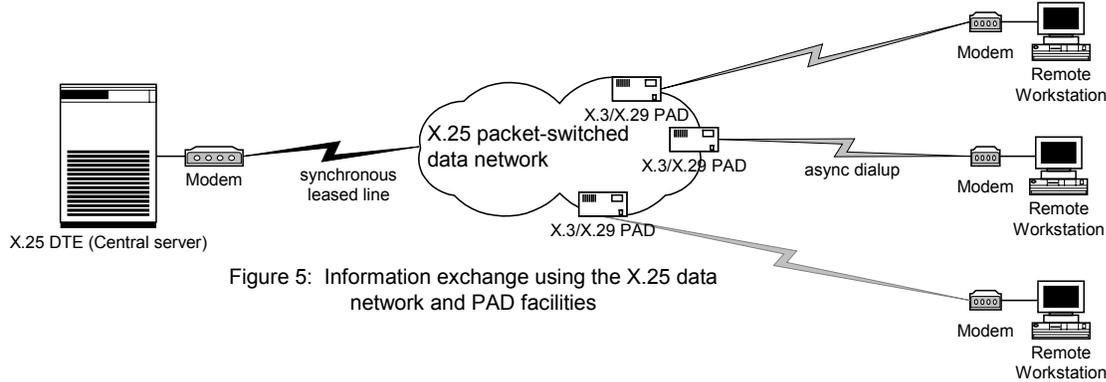
Figure 5: Information exchange using the X.25 data network and PAD facilities
