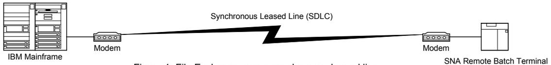
Figure 1 illustrates a point-to-point network connection for file exchange with IBM mainframes. A synchronous frame-switching approach is the easiest migration for this type of connection, since the software for terminal devices and host applications is usually not amenable to change. In a frame-switching environment, the IP interface/switching devices have no knowledge of the protocol running over the synchronous leased line illustrated in the diagram.
